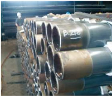
Fusion Bond Epoxy Coating (FBE)
