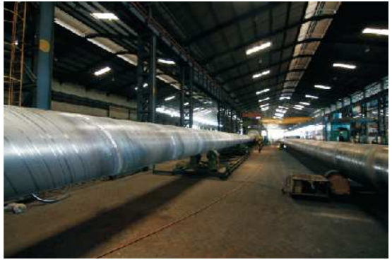
Spiral Pipe Manufacturing Process Length : 72 m, without connection
