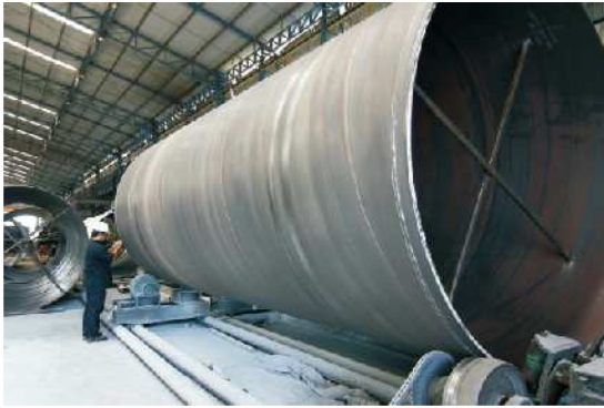
Spiral Pipe Manufacturing Process Diameter width : 3.2 m
