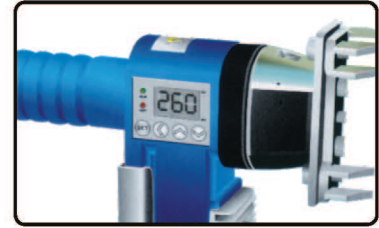
3. Heat the welder to 260°C
